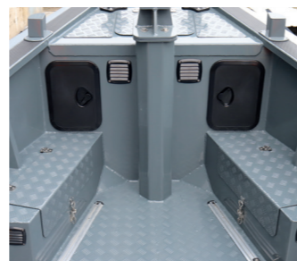
Storage lockers in the bow with quick-access hatches for storage
