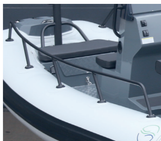
Additional railings on tubes
