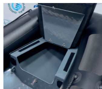
Built-in ventilated bow locker with an antiskid coating, where you can place a 12-liter fuel tank.
